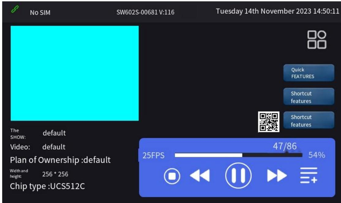
At the top of the interface is the network signal, controller ID number and the date, time and device software version display
