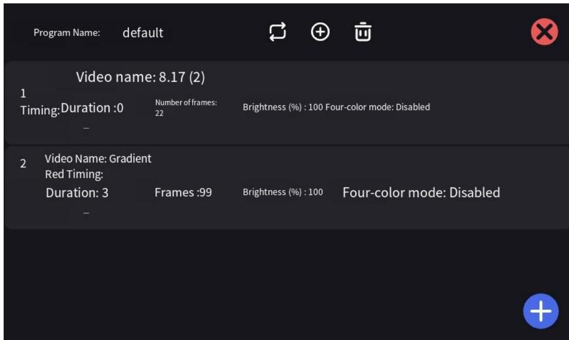
Controller factory prefabricated a program, program name is the default. It can be operated by the icon on the back
